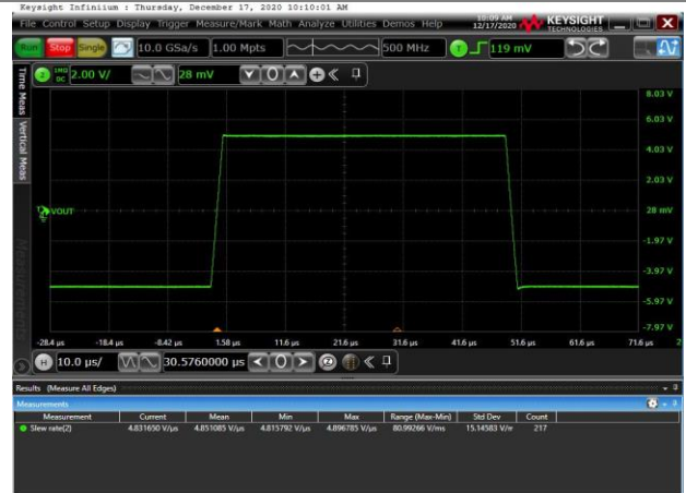
Voltage: 2V/div for Output, Time: 10us/div G=1, VREF = GND; VIN=10VPP, Load R=10K Figure 20 Slew Rate
