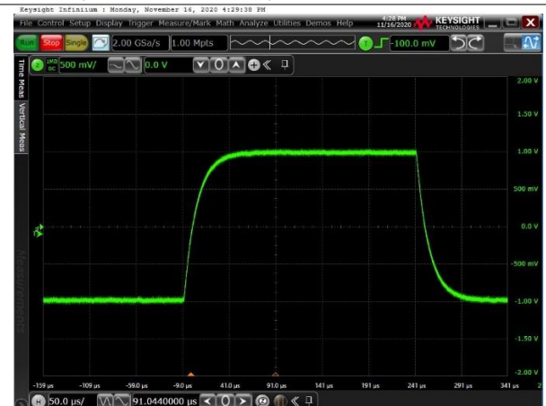
Voltage: 500mV/div for Output, Time: 50us/div G=10, VREF = GND; VIN=2mVPP, Load R=10K C=100pF
