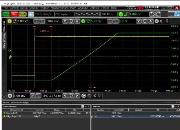
Voltage: 5V/div for Output, Time: 2us/div G=10, VREF = GND; VIN=10VPP, Load R=10K C=100pF Figure 21 Positive Overload Recovery
