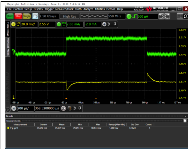
Figure 13. Load Transient, \pm 2 mA, V_{IN} = 5 V, C_{IN} = 1 \mu F, C_{OUT} = 1 \mu F, 20 mV/div
