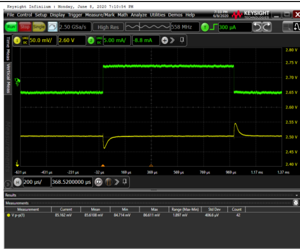
Figure 11. Load Transient, \pm 5\text{ mA} , V_{IN} = 5\text{ V} , C_{IN} = 1\text{ }\mu\text{F} , C_{OUT} = 1\text{ }\mu\text{F} , 50 mV/div
